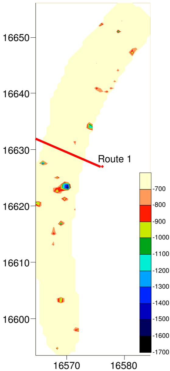
**Figure I.11: 2-Dimensional Contour Plot of Magnetic Deviation Acquired from the Site Survey. Data Range from -700 nT to -1700 Nt on a Background of -600 nT**
