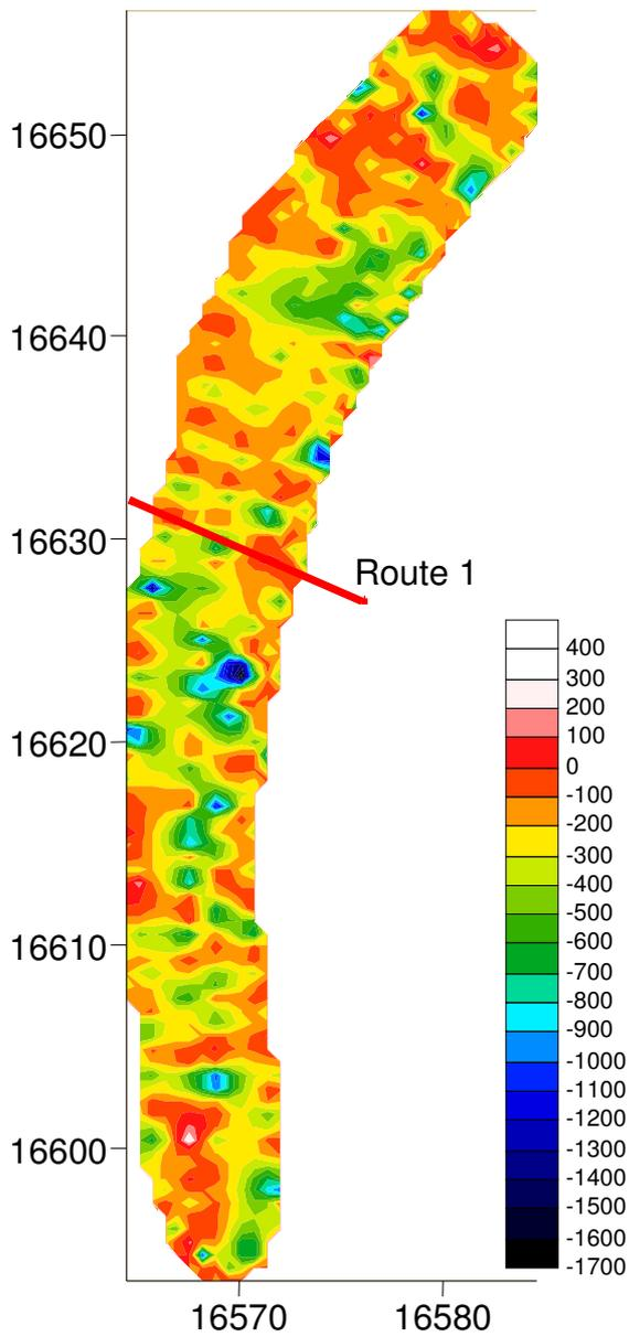
**Figure I.10: 2-Dimensional Contour Plot of Magnetic Deviation Acquired from the Site Survey. Data Range from +400 nT to -1700 Nt on a Background of 300 nT**
