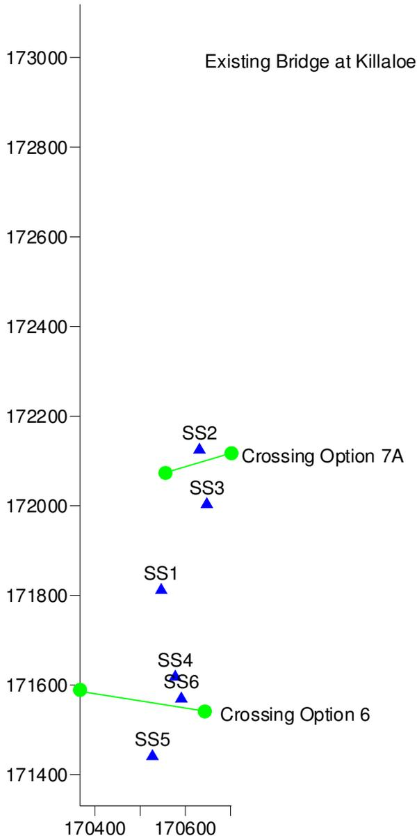
**Figure I.19: Location of the Anomalies Interpreted from the Sidescan Record in Relation to the Proposed Crossings (Scale to Irish National Grid)**
