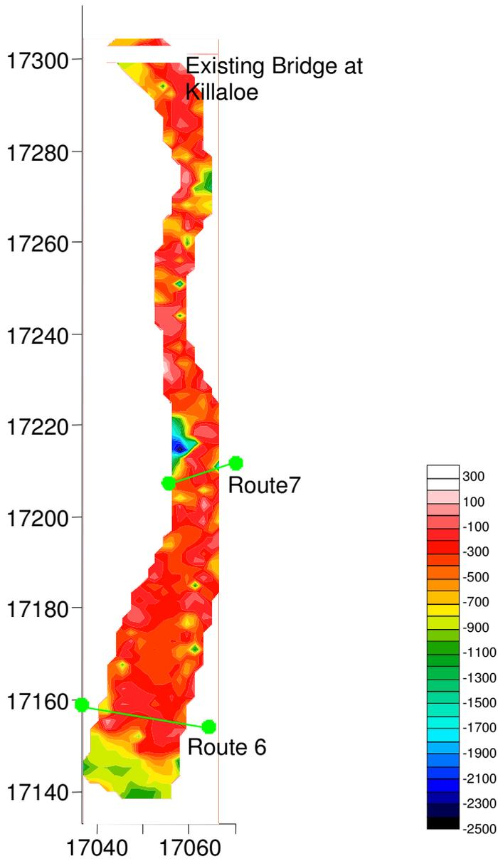
**Figure I.7:** 2-Dimensional Contour Plot of Magnetic Deviation Acquired from the Site Survey. Data Range from +300 nT to -2500 Nt on a Background of -200 nT
