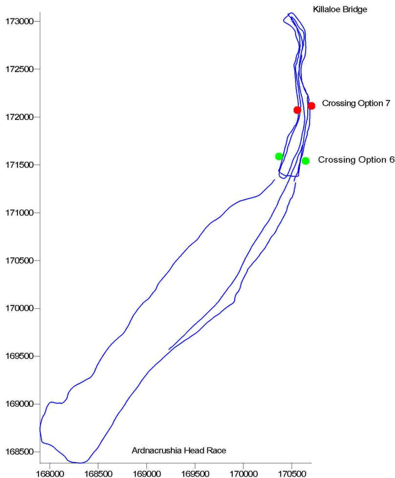
**Figure I.1: Track chart resulting from site surveys at Killaloe/Ballina (Scale to Irish Grid, Ireland 65 Datum).**
