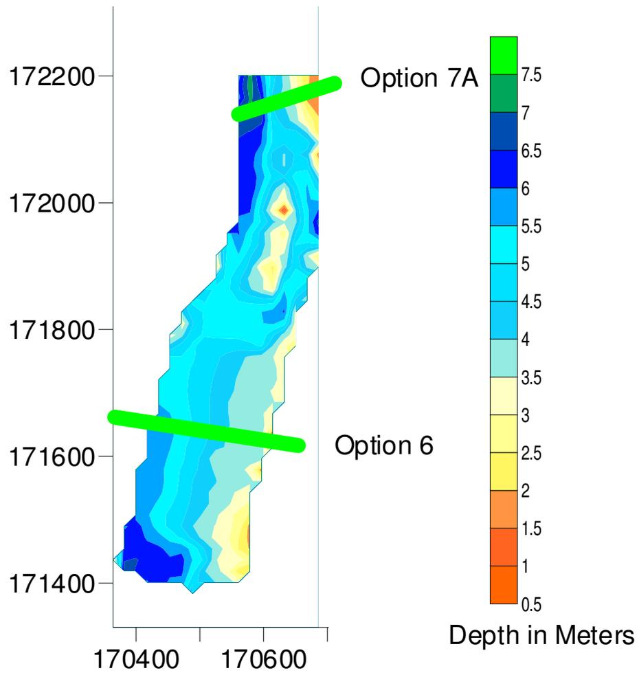
**Figure I.5: 2-Dimensional Contour Plot of Bathymetric Data Obtained at and Adjacent to the Zone of Proposed Impact at Killaloe/Ballina**
