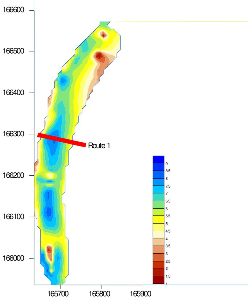
**Figure I.6: 2-Dimensional Contour Plot of Bathymetric Data Obtained over the Study Area at O'Briensbridge/Montpelier**
